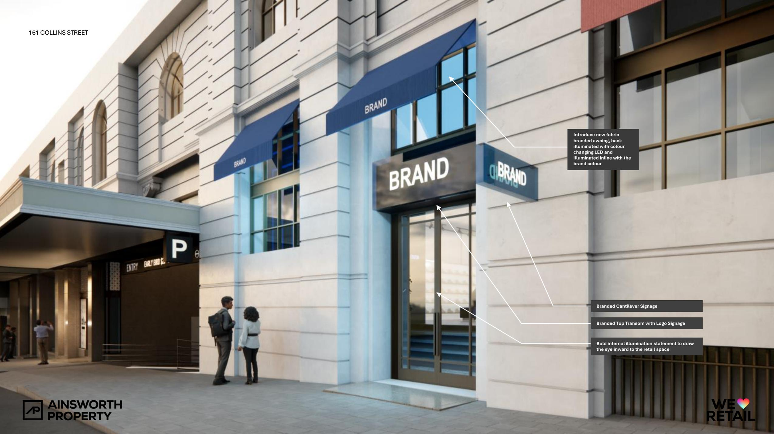
Introduce new fabric branded awning, back illuminated with colour changing LED and illuminated inline with the brand colour
